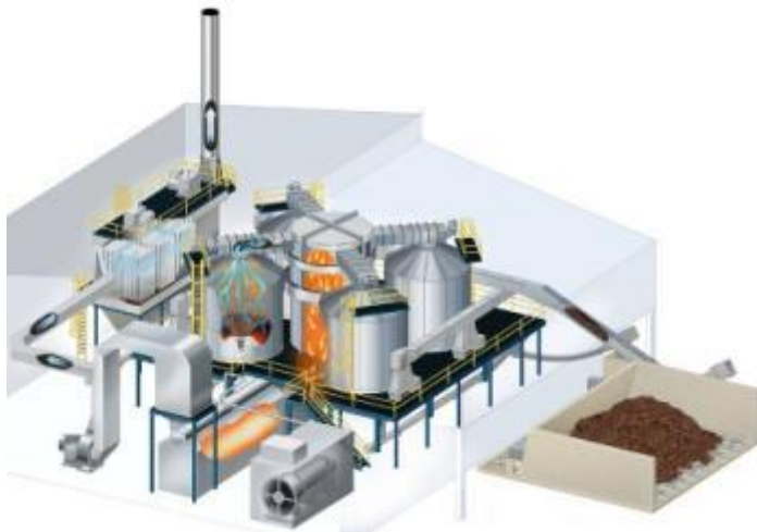
Greenfield - Gasification to steam power or steam CHP Standard configurations from 2 – 10 MWe
